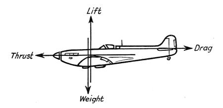
The thrust is provided by the propeller, EDF, etc., whilst the drag is the air resistance to the aircraft moving through the air. The lift is provided by the airflow over the wings while the weight shown acts through the centre of gravity of the aircraft in its flight mode.
